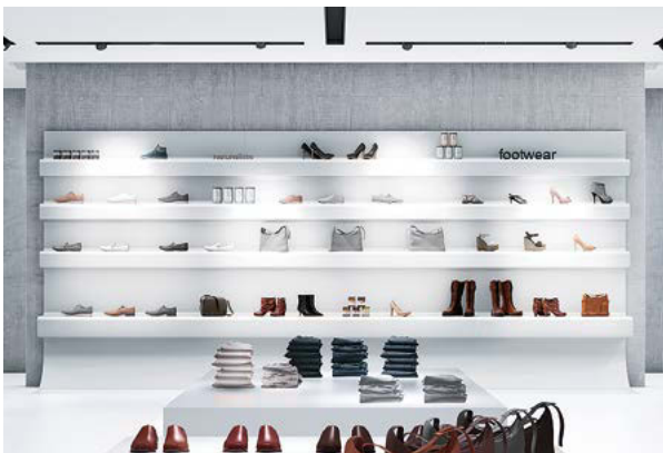
Previously: several round to oval lighting cones used to illuminate vertical surfaces only in selective areas, leaving dark zones.
