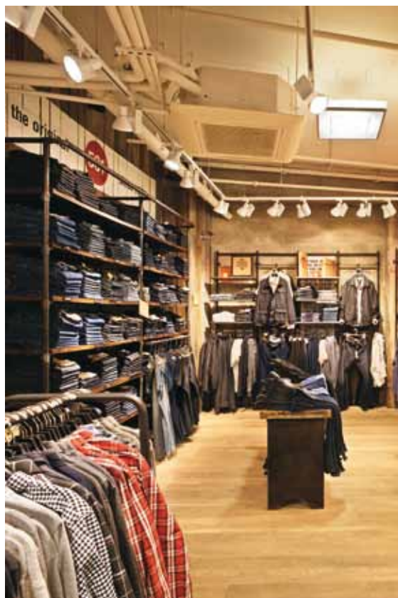
B4 | Visible technology: the lighting suspension system is fully visible. Instead of being conceived as a fault, this lack of coverage complements the robust image of the shop. The spotlights can be arranged flexibly as required. Pleasant basic illumination is provided by four square LED light fields.
